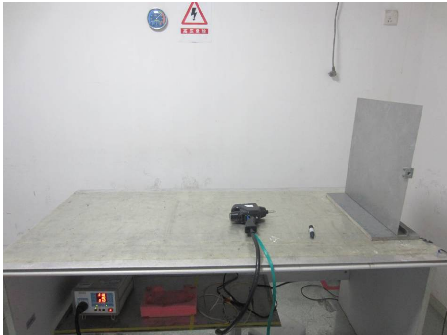
ESD Test Setup Photograph
